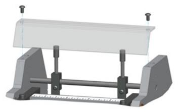
2. Loosen output shaft set screws (x2) and partially slide output shaft out, while removing only one existing output guide from the shaft (do not remove shaft completely). Install new center output guide(s) on output shaft. Additional center output guide(s) must always be installed between the original "outside" output guides that came with the unit (Note orientation of "outside" output guides as they are specific to each side and are not reversible).
